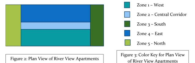
The division of zones shown above allows for simple block load analysis to be performed. River Vue Apartments is rotated approximately twenty degrees off true north on its building site. This rotation influences the solar gain seen by each zone and was taken into account in the Trane TRACE model for accuracy.
